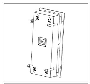
2step: Use the screw in the package to fit the CK-650 into the wall
