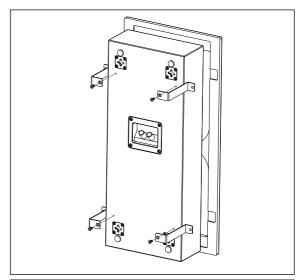
2step: Use the screw in the package to fit the CK-450 into the wall
